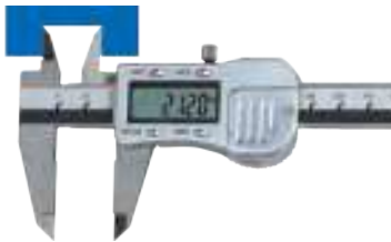
Innenmessung / internal measuring
